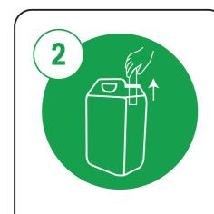
Remove the Chemical Pick Up tube from the empty container
