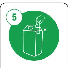
Insert the Detergent Chemical Pick Up Tube
