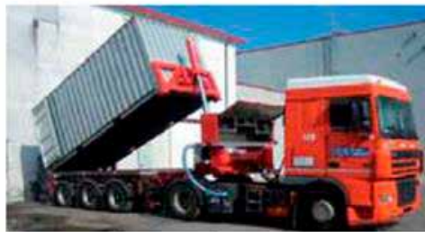
Container trucking - linerbags and rotary valve
